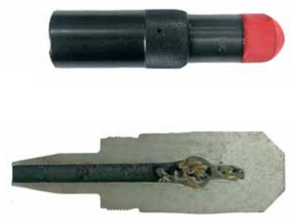
Cutway View After Receiving Three Bullets
